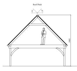
To make best use of edges and corners of the upper floor, OakCraft's unique extended eaves option allows up to 1.2 metres vertical extension.
